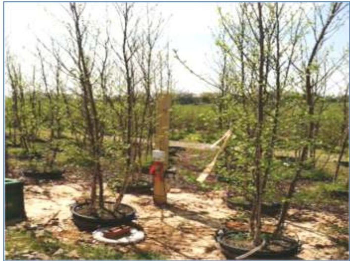
Fig. 48. Birch block single node installation, with the three sensed trees and tipping rain gauges monitoring irrigation applications and leaching (white bucket in foreground).
