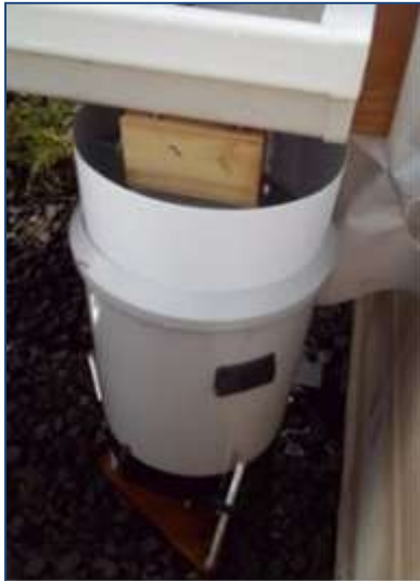
Fig. 13. Nested rain gauges measuring runoff from each green roof platform
