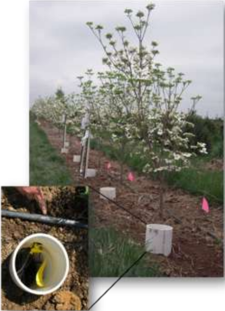
Fig. 44. Decagon EM50R network on Cornus florida trees at Raemelton Farm. Insert shows sensors located in PVC tube in the root zone.
