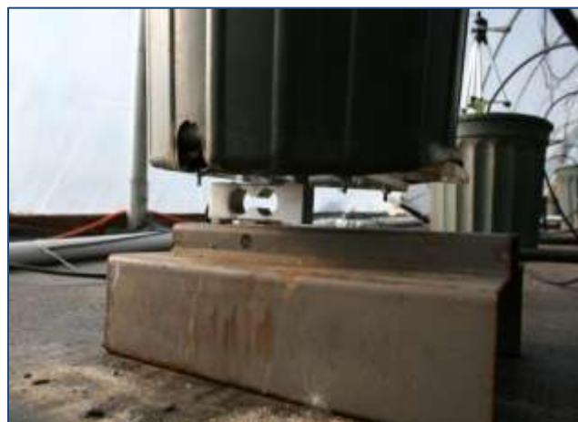
Fig.25. A close up of a pot mounted on a load cell. Load cells allowed us to weigh the plants automatically twice a day. Those weights were then used to calculate daily water use.
