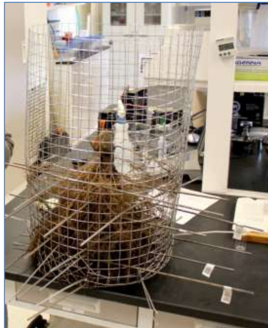
Fig. 36. Example of a tree root system that had been CT scanned over a growing season. Soil was removed using an air spading technique. The roots were held in original locations using artificial scaffolding.
